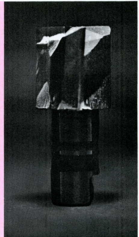
LEFT — A machined metal part as it looks under ordinary general lighting. RIGHT — Under black light, glowing fluorescent dye reveals a crack in the same part which at left looked like an acceptable part under ordinary light.
